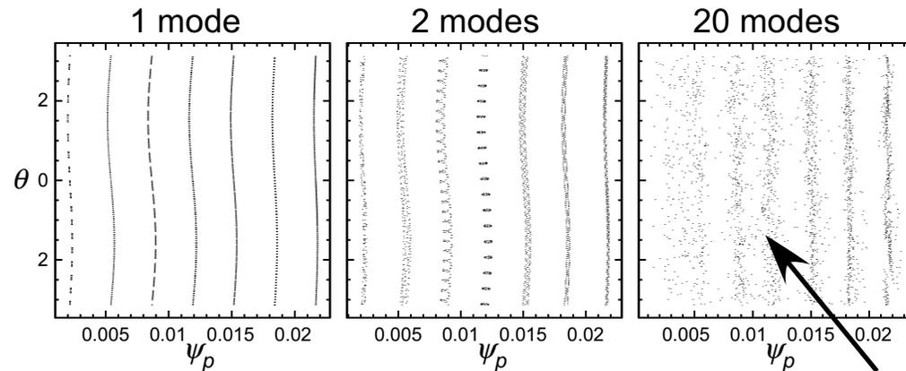
Poincaré plot of electron trajectory
