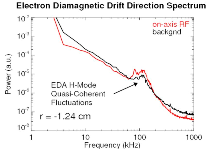
Shows density fluctuations in SOL diminish during on-axis heating
