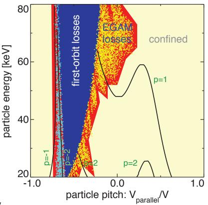
blue dots: lost particles that give >1% of its energy to the mode yellow dots: lost particles that gain >1% of its energy from the mode
