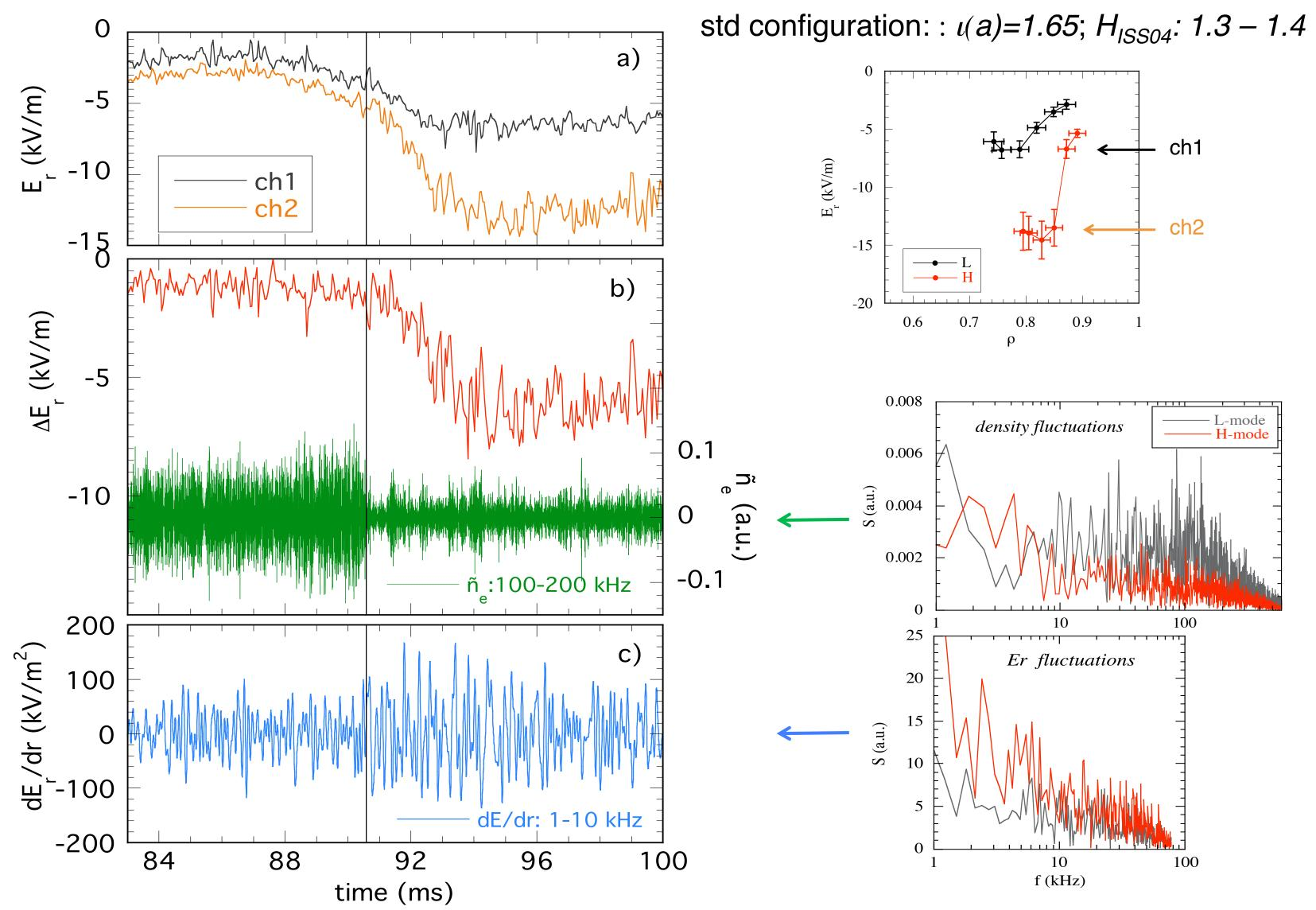
At the L-H transition the turbulence reduction precedes the increase in the mean
